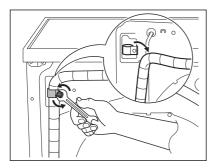
4. Put the end of the drain and inlet hose in a container. Let the water flow out of the hoses.
