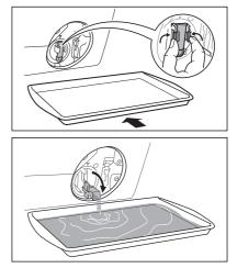
3. When the container is full of water, put the drainage duct back again and empty the container. Do step 2, 3 again and again until no more water flows out from the drain pump.
