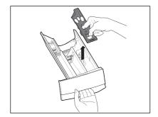
Flush it out under a tap to remove any traces of accumulated powder.
