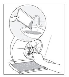
4. Push back the drainage duct and turn the filter counter-clockwise to remove it.
