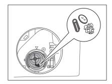
6. Make sure that the impeller of the pump can turn. If this does not occur, contact the service centre.
